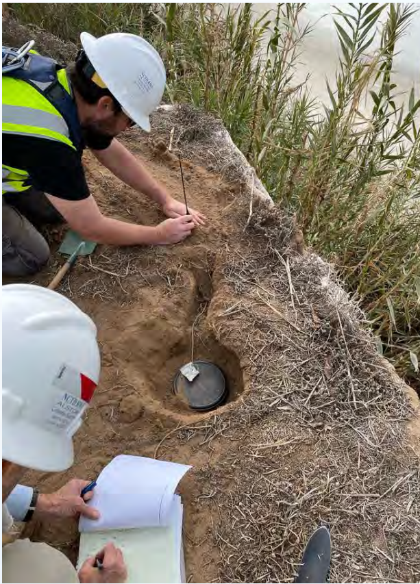
(Left) In-ground sensor installation in Del Mar. (Right) cliff top cracks and sensors at San Elijo State Beach and a total station cliff survey at Beacon's.
