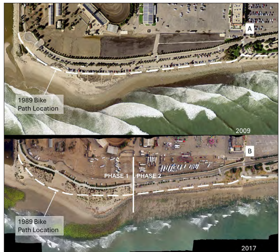
Figure 5. Aerial photographs Surfers Point Phase 1 (A) before (2009) and (B) after (2017) construction. The solid line indicates the seaward edge of development before construction. Source: 2009 imagery collected by USACE; 2017 imagery collected by Sierra Overhead Analytics.
