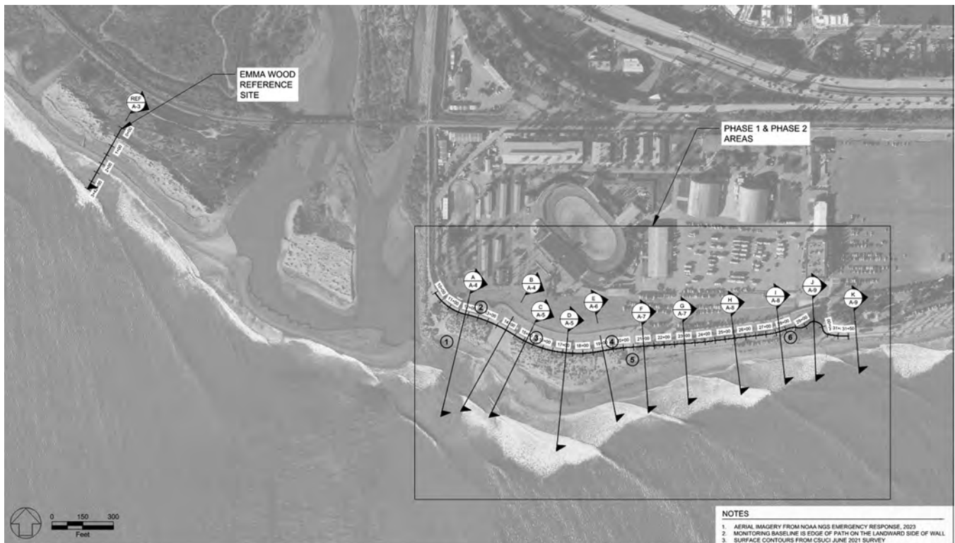
Figure 10. Elevation survey transects (Profiles A-J and REF) at Surfers Point Phase 1 (A-E), Phase 2 (F-J) and the Emma Wood reference Site (REF). The shore-parallel line is a station line along the new pedestrian path. Source: ESA et al. 2024.
