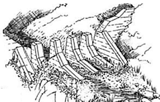
Figure 3-6. Debris Flow Breaker.
