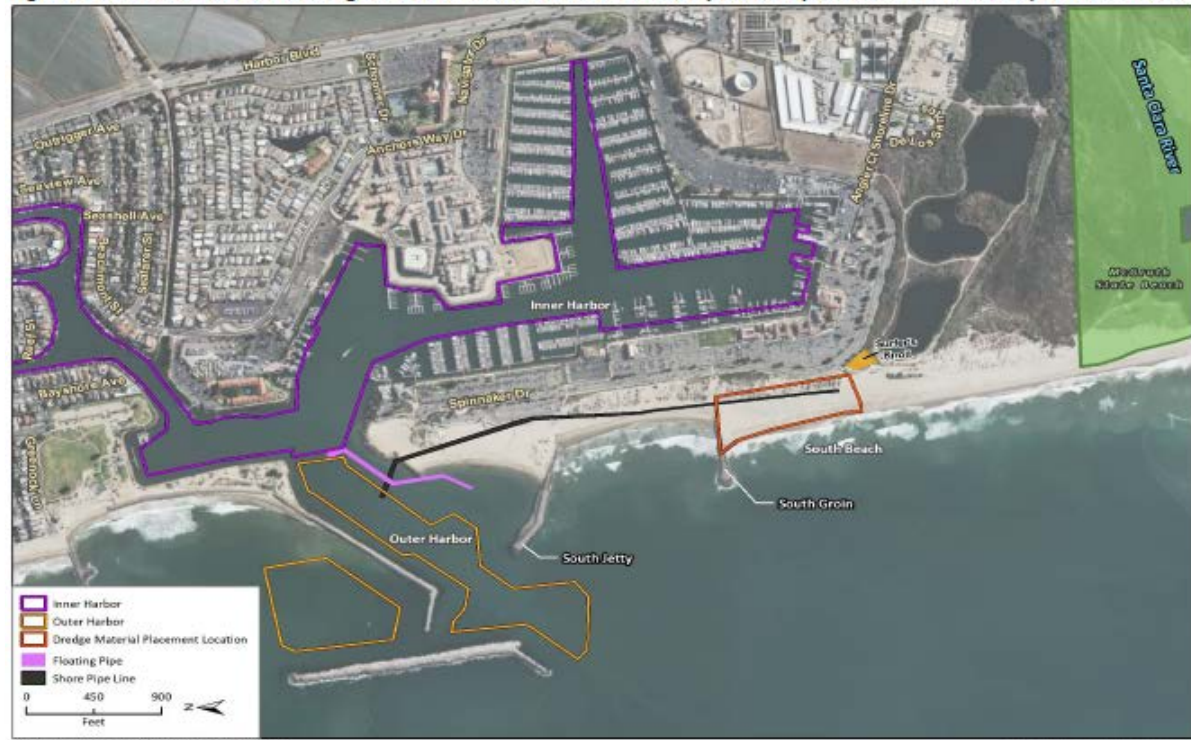
Figure 2. Ventura Outer Harbor Dredge Material Placement Location and Pipelines Implemented from February to March 2022
