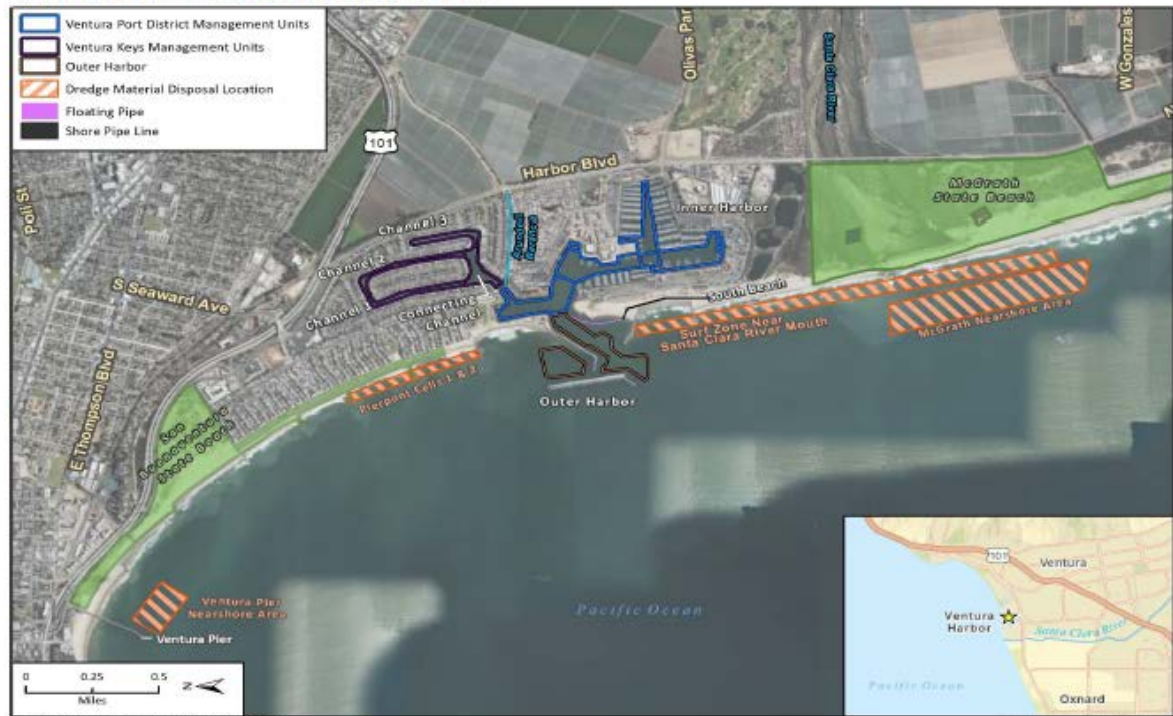
Figure 1. Ventura Harbor Maintenance Dredging Regional Location with Inner and Outer Harbors Maintenance Dredging Areas and Approved Dredge Material Placement Locations
