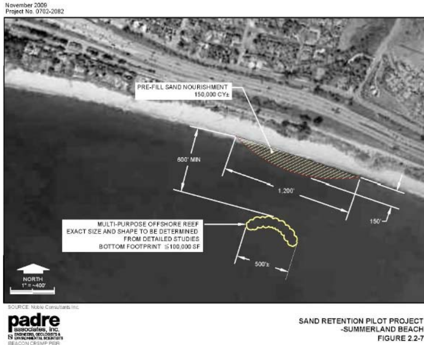
This figure shows a typical 'Multi-purpose Offshore Reef' design from the BEACON CSMP.
